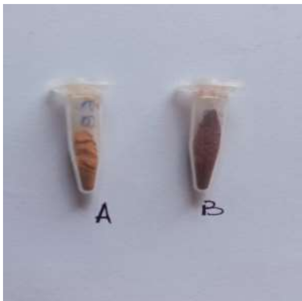
Figure 1. The color change of Butea monosperma flower extracts before and after synthesis of silver nanoparticles. (a) The flower extract of Butea monosperma (yellow) and (b) \text{Fe}_2\text{O}_3 - Butea monosperma emulsion after 24 h (reddish brown).
